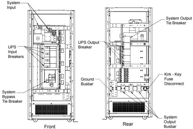
Figure 44 Liebert<sup>®</sup> NX<sup>™</sup> 480V paralleling cabinet with input and bypass circuit breakers, main components
